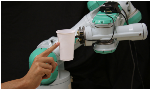
Figure 2.10: A human-robot grip stabilization experiment where a human and a robot collaborate in order to preserve a stable grip on a deformable plastic cup. Image taken from [6].
